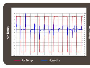
ADI® technology is being tested under extreme temperatures (-40 to +70 degrees C) and humidity approaching saturation points (90+%). This ongoing test, which is approaching two years in duration, is yielding favorable results that confirm measurably extended lifecycle of the product.
