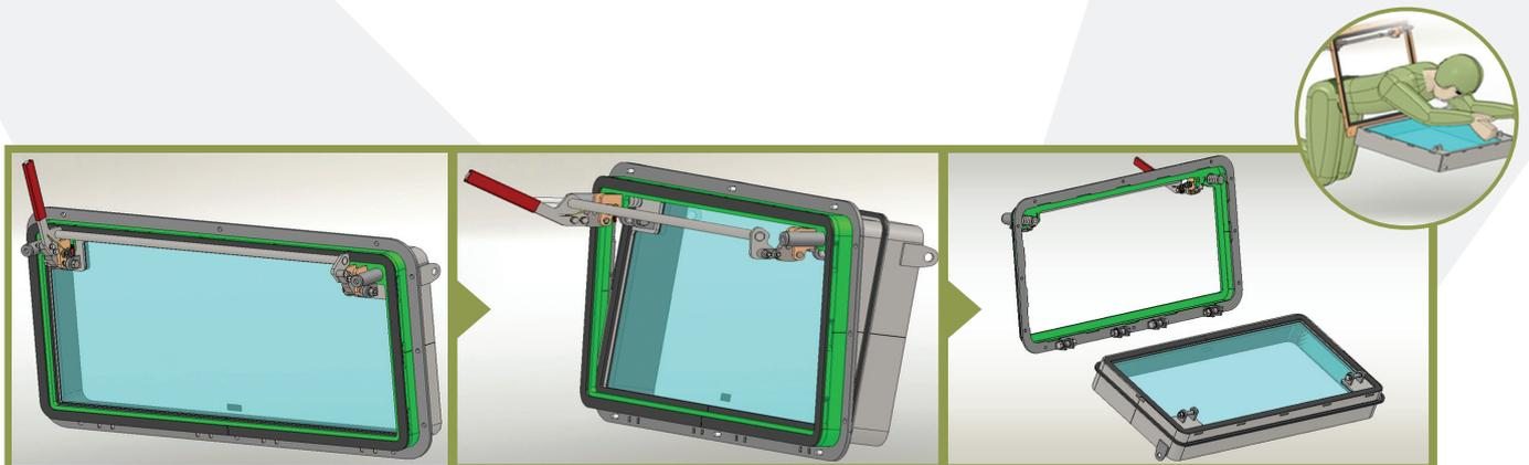
OSG's EEWS solution operates efficiently regardless of vehicle position, offering egress route when doors are blocked.
